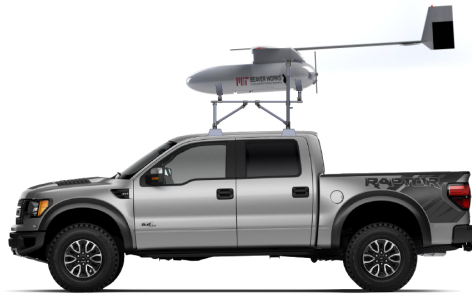
Figure 2: The aircraft is mounted on the back of a launch vehicle, which brings the aircraft to rotation speed.
