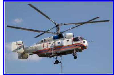
(f) An example coaxial helicopter: the Kamov Ka-32 [28].
