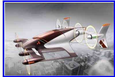
(c) An example tilt wing aircraft: the A 3 Vahana [25].
