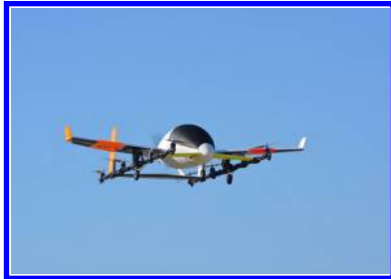
(a) An example lift + cruise aircraft: the Aurora Flight Sciences prototype [23].
